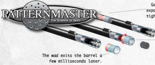
Gases from the burning powder expand the wad base to create a tight seal, then propel the wad down the barrel.
